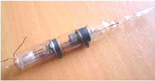
Fig. 1. Metal-glass construction of SRNV-1.
